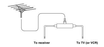
Connecting the antenna cable to the 75/300  $\Omega$  antenna adapter (For all models other than European models)
